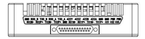
The interface of the device adopts J30J-25pin. The interface consists of 1 power supply, 2 RS232/TTL, 1 RS422, 2 SBUS or 1 TTL, and 2 Ethernet ports.
