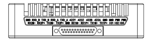
The interface of the device adopts J30J-25pin. The interface consists of 1 power supply, 2 RS232/TTL, 1 RS422, 1 SBUS/TTL, and 2 Ethernet ports.
