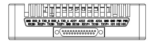
The interface of the device adopts J30J-25pin, and the interface has a total of 1 power supply, 2 RS232, 1 RS422 and 2 network ports.
